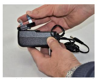
10. Attach the correct fitting to the power adaptor for your country [PHOTO] and plug this into an electrical socket. The Bubble Column is now ready for use.
