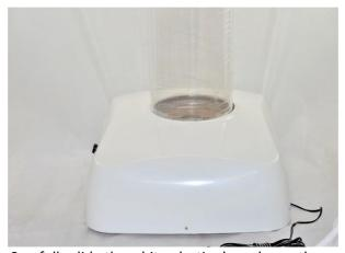
8. Carefully slide the white plastic shroud over the column to cover the base. The bubble pattern selector needs to be 'eased' through the hole in the shroud.
