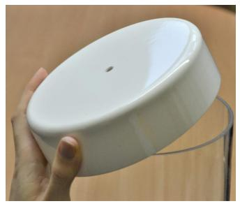
1. Remove the white plastic cap found at the top of the bubble column.
